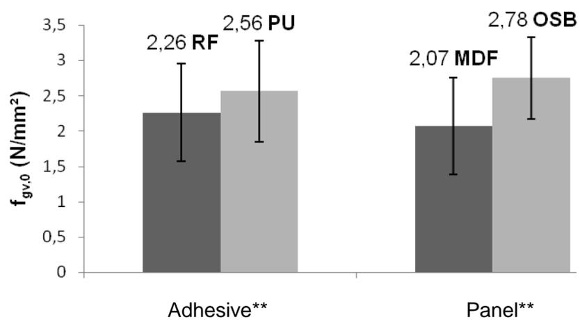
**Figure2** –Effect of adhesives and panels in the glue line shear strength.
