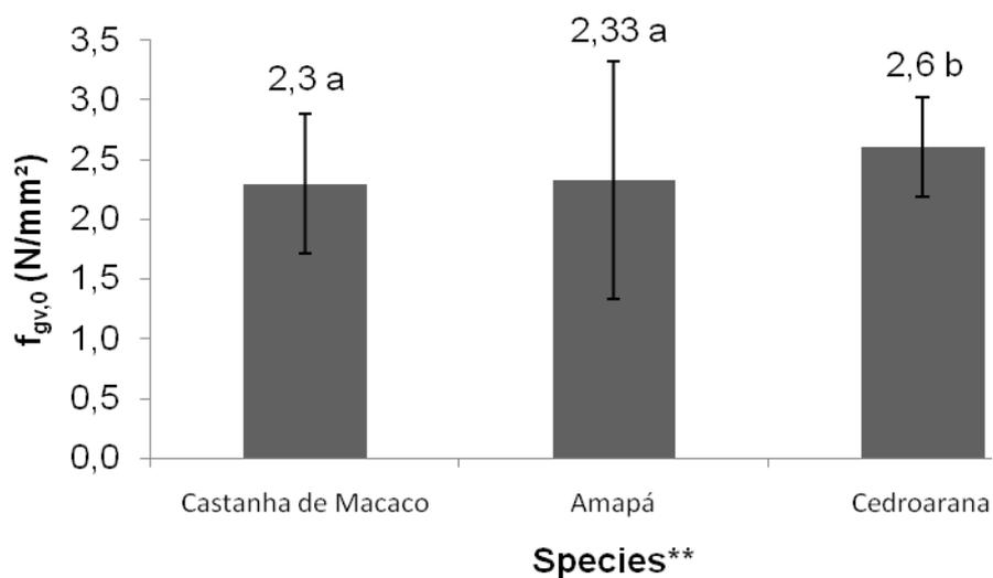
**Figure 1**–Effect of species on the tensile strength. (\*\* Means followed by same letter do not differ statistically by Tukey test at 1% significance).
