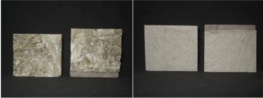
**Figure 3** – Inner surface aspect of the samples - Failure on OSB panel (left) and failure on MDF panel (right).
